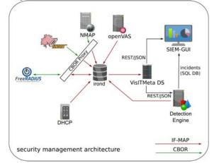
Figure 2: Management architecture of the demonstration
