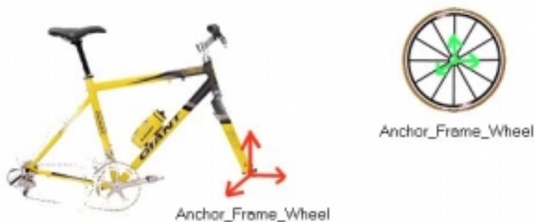
**Figure 9: Anchors for the assemblage between a frame and a wheel**
